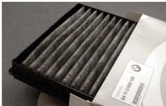
*The interval for cabin air filter replacement varies according to the conditions the car lives in, so do frequent visual inspections.*
