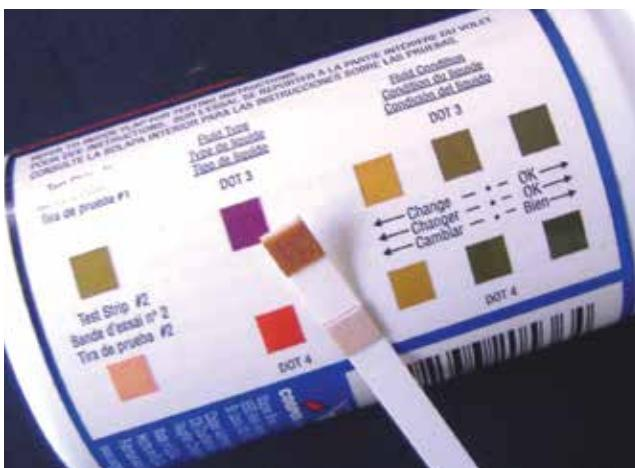
*A visual indication of the need for brake fluid changes can be provided by test strips, which can be stapled to repair orders. A flush and change every two years is recommended.*
