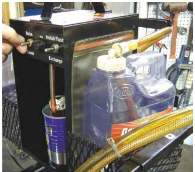
*Although you can do a power steering fluid flush/refill without one, a relatively inexpensive purpose-built flushing machine will make the procedure faster, neater, and more complete. Use the right stuff!*
